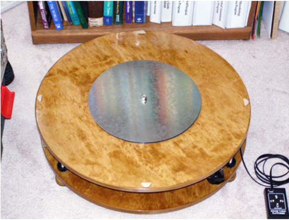
Platform prepared to receive the dob base with bearing and felt pads.
