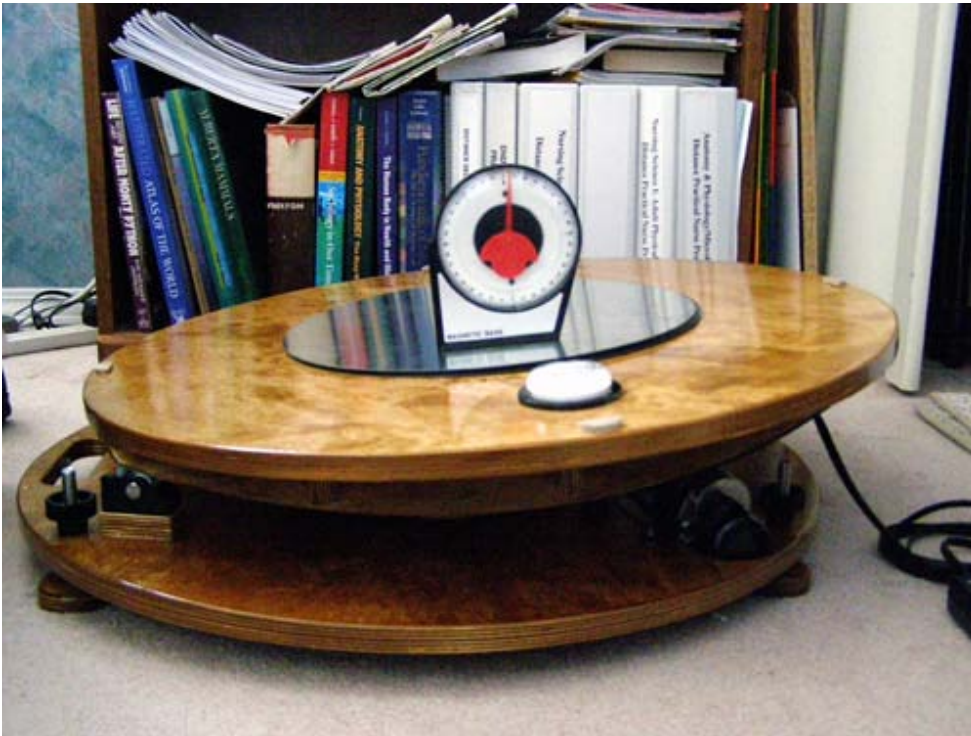
Test run, measuring angle tilt, time and wobble....no wobble, runs for 52 minutes before motor is automatically stopped. Lever is engaged, and platform rolled back, lever engaged and tracking is resumed.
