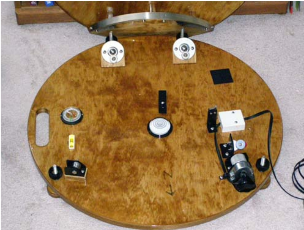
Detail of base with bearings motor, compass etc.
